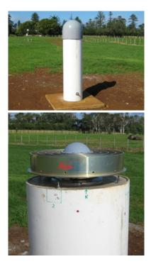
**Figure 1.** Typical AuScope GNSS installation at Norfolk Island collocated with Australian Tsunami Warning Service (ATWS) seismograph station.
