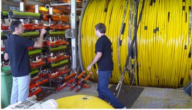
Figure 1. The 8 kilometre solid streamer, tail buoy and stabilizer 'birds' being inspected prior to the start of the Southwest Margin 2D seismic survey.
