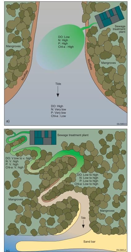
Figure 3 (a) and (b). Conceptual diagrams of Myrmidon and Buffalo Creeks showing geomorphology, sewage discharge points and nutrient and oxygen conditions.
