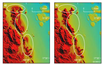
**Figure 3.** False-colour images showing the reduction to the interpolation artefacts between the continental shelf and land areas using the improved interpolation process. Comparison of the 2005 version of the grid (a) and the 2009 version (b) with variations highlighted by circled areas.
