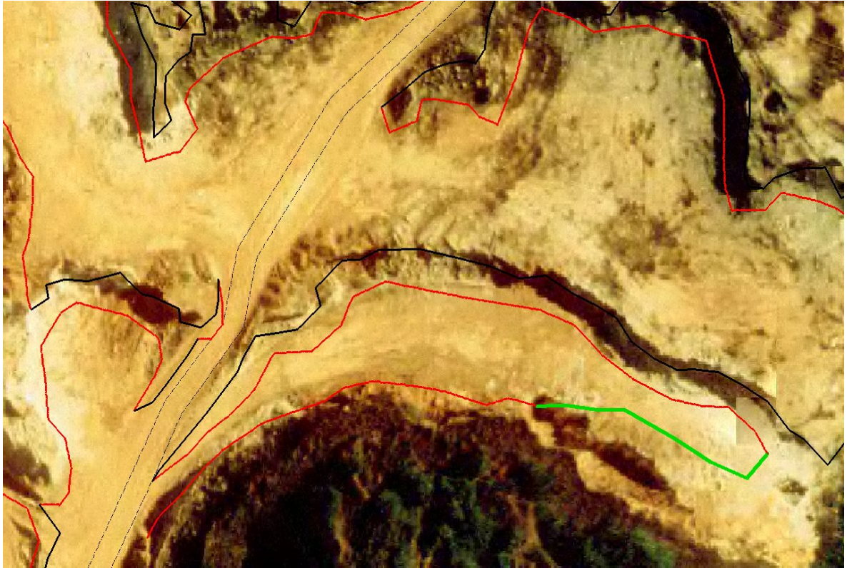
Figure 34: An example of some survey pick up of toe lines (in red) and crests (in black). The track survey pick up is grey.
