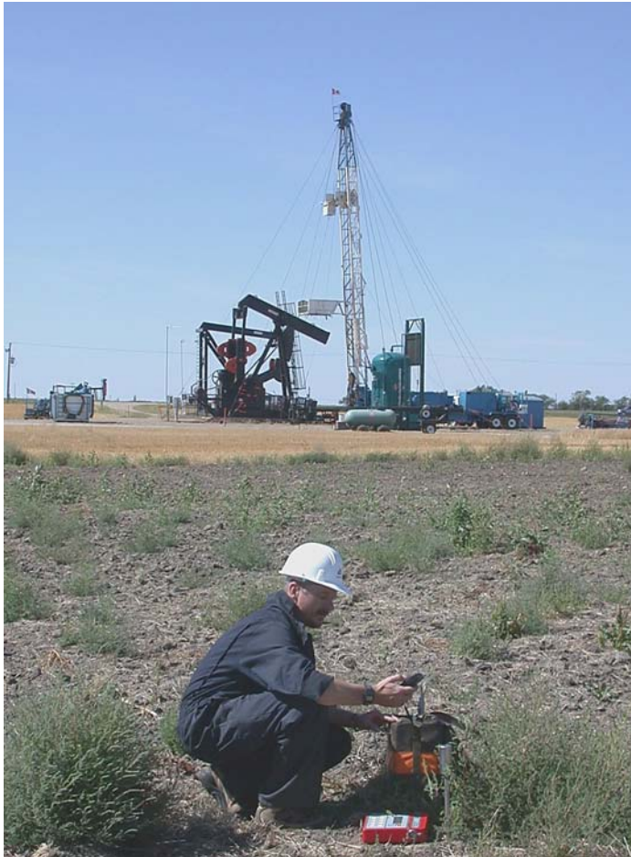
Soil gas measurement in the Phase 1 CO 2 injection area of the Weyburn oilfield. Note the in-situ soil gas probe to the right of the portable gas analyzer (red).
