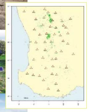
Figure 1. The red dots show the GPS stations that were 'occupied' for a week in May. The green dots indicate known earthquakes in the region.
