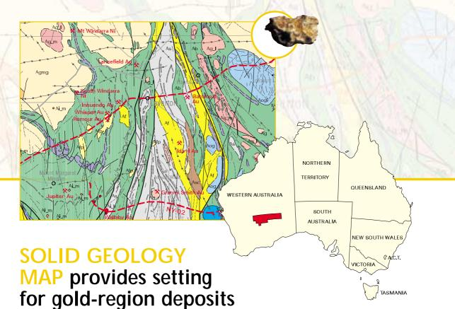
Geoscience Australia's new, solid geology map of the Leonora to Neale region in the Eastern Goldfields of Western Australia is an initial step towards developing a 3-D model of the area, and provides a basis for analysing seismic reflection lines acquired in 2001.
