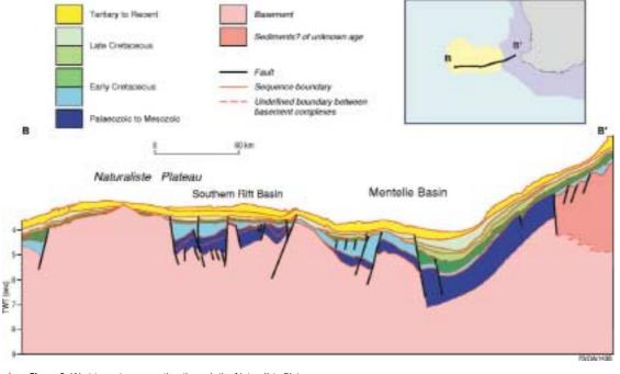
Figure 3. West to east cross-section through the Naturaliste Plateau based on interpreted Shell 'Petrel' seismic line, N325
