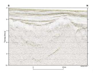
Figure 1. Part of a seismic line from the deep-water margin of George V Land, Antarctica, acquired during Geoscience Australia's latest survey on the Geo Arctic. The sediments in the top of the section were deposited during the separation of Australia's and Antarctica during the past 80 million years. In this section the sediments are about 1500 metres thick. The reflectors in the bottom of the section come from the crust at a depth of about 14 kilometres.
