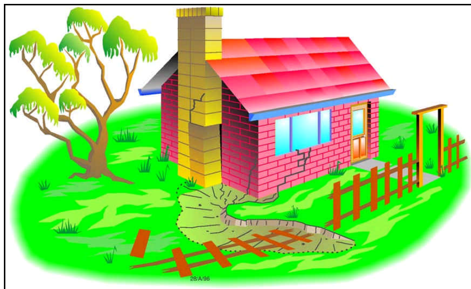
Figure 3.14 Schematic diagram representing cracks in masonry and tilting fences due to ground subsidence.
