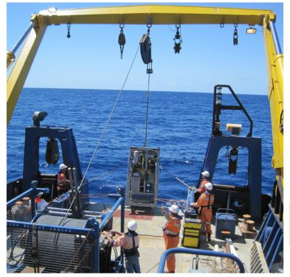
**Figure 1.** The remotely operated vehicle being deployed from the Australian Government's Marine National Facility the RV *Southern Surveyor* during the marine survey searching for evidence of natural hydrocarbon seepage sites in the offshore northern Perth Basin. The RV *Southern Surveyor* is owned and managed by CSIRO.
