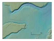
**Figure 4.** High resolution multibeam sonar image of the seafloor on the outer continental shelf of Joseph Bonaparte Gulf showing pockmarks formed in muddy sands across a valley floor.
