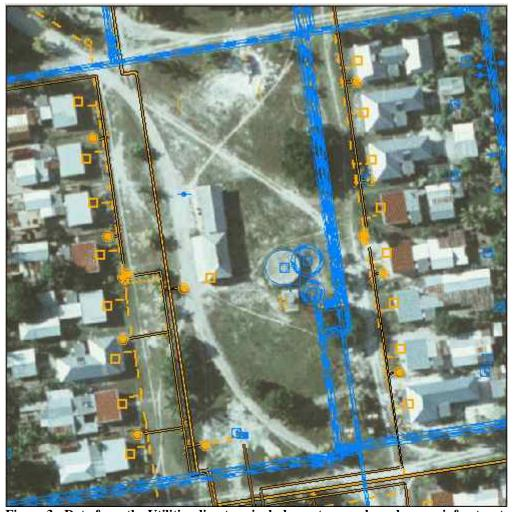
Figure 3: Data from the Utilities directory includes water supply and power infrastructure points, lines and polygon.
