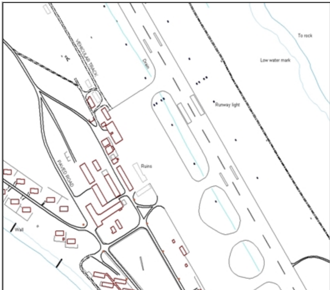
Figure 3. An example of AUSLIG topographic data around the airport. The dataset also has elevation data including contours and spot heights and some incomplete polygon data.
