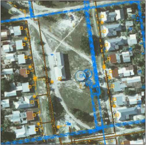
Figure 27: Data from the Utilities directory includes water supply and power infrastructure points, lines and polygon.
