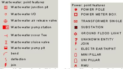
Figure 28: Examples of utilities legends in ArcView after installation of the font containing the GHD symbol set.
