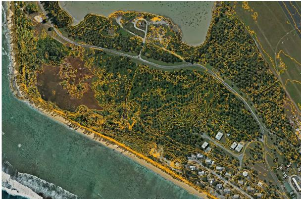
Figure 23: Sample of 0.5m contours generated from the 2011 digital elevation model.
