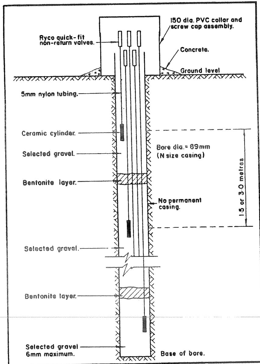
Figure 29. Borehole salinity monitoring system.
