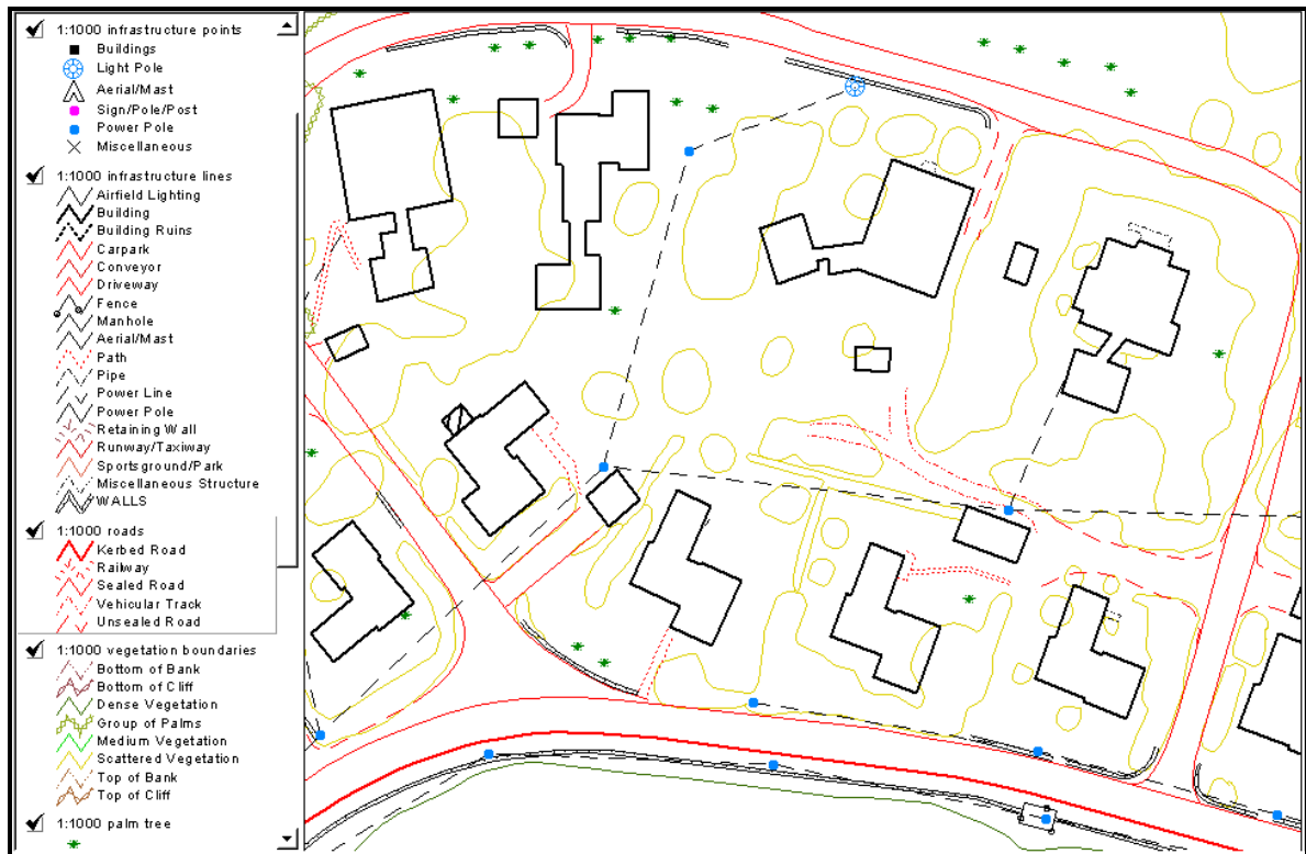
Figure 32: Screen capture of part of Rocky Point showing typical line and point features of the 1:1000 detail survey data. This data was digitised directly from the 1987 aerial photography so when compared to the orthophotography it matches very well.
