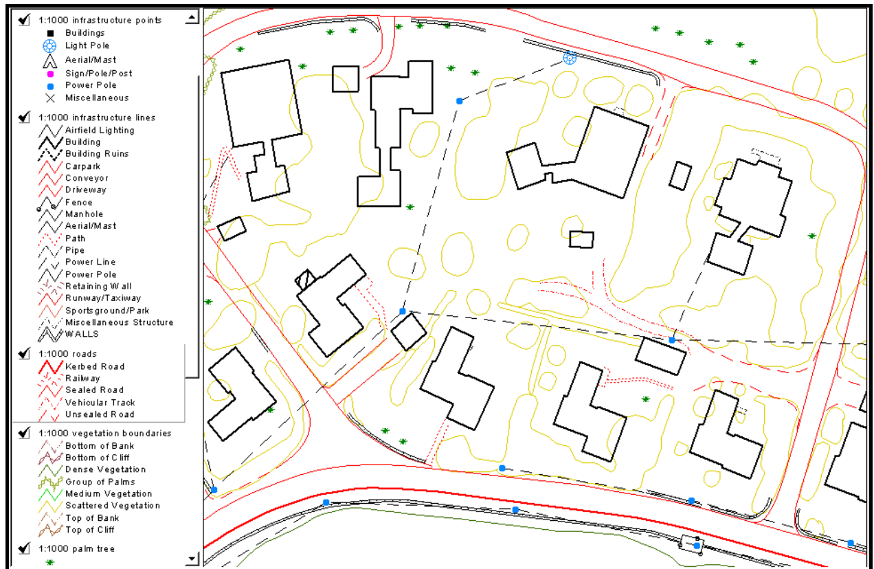
Figure 49: Screen capture of part of Rocky Point showing typical line and point features of the 1:1000 detail survey data. This data was digitised directly from the 1987 aerial photography so when compared to the orthophotography it matches very well.
