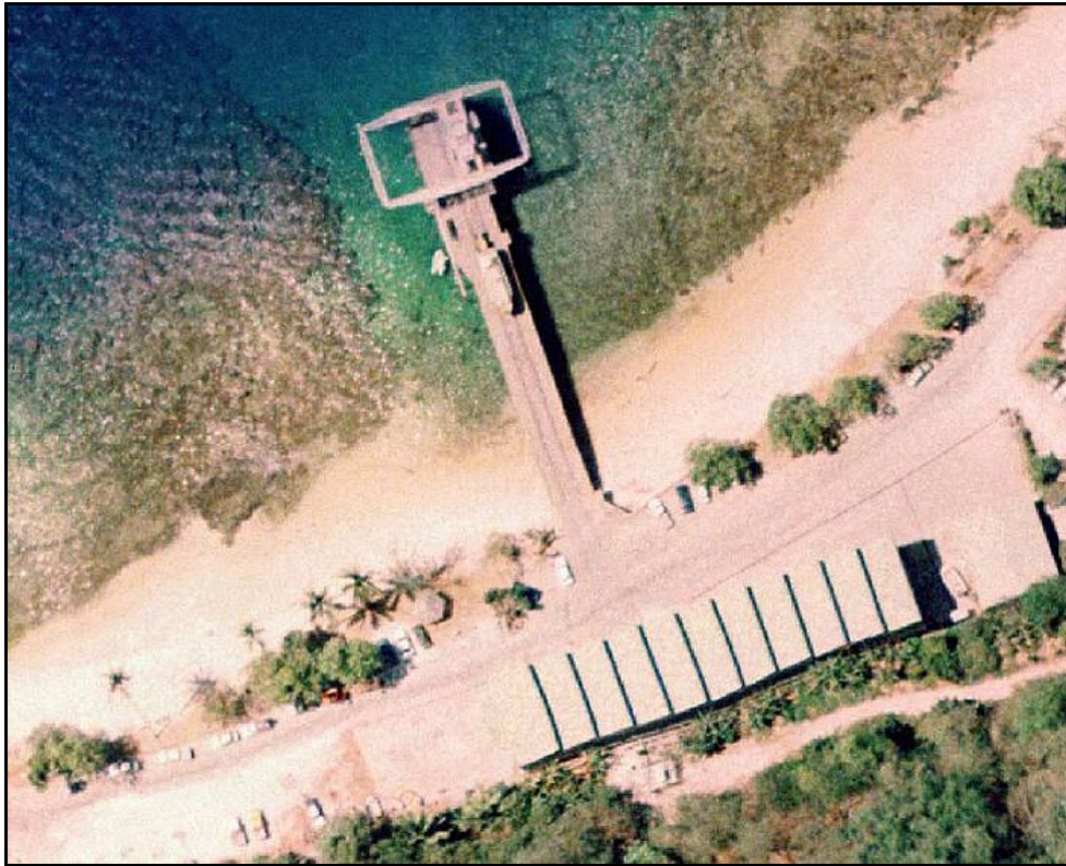
Figure 18: An image captured from the Christmas Island GIS orthophotography at approximately 1:800 scale, showing clarity and resolution of land and underwater features. The current orthophotography was created from aerial photography flown in 1997.
