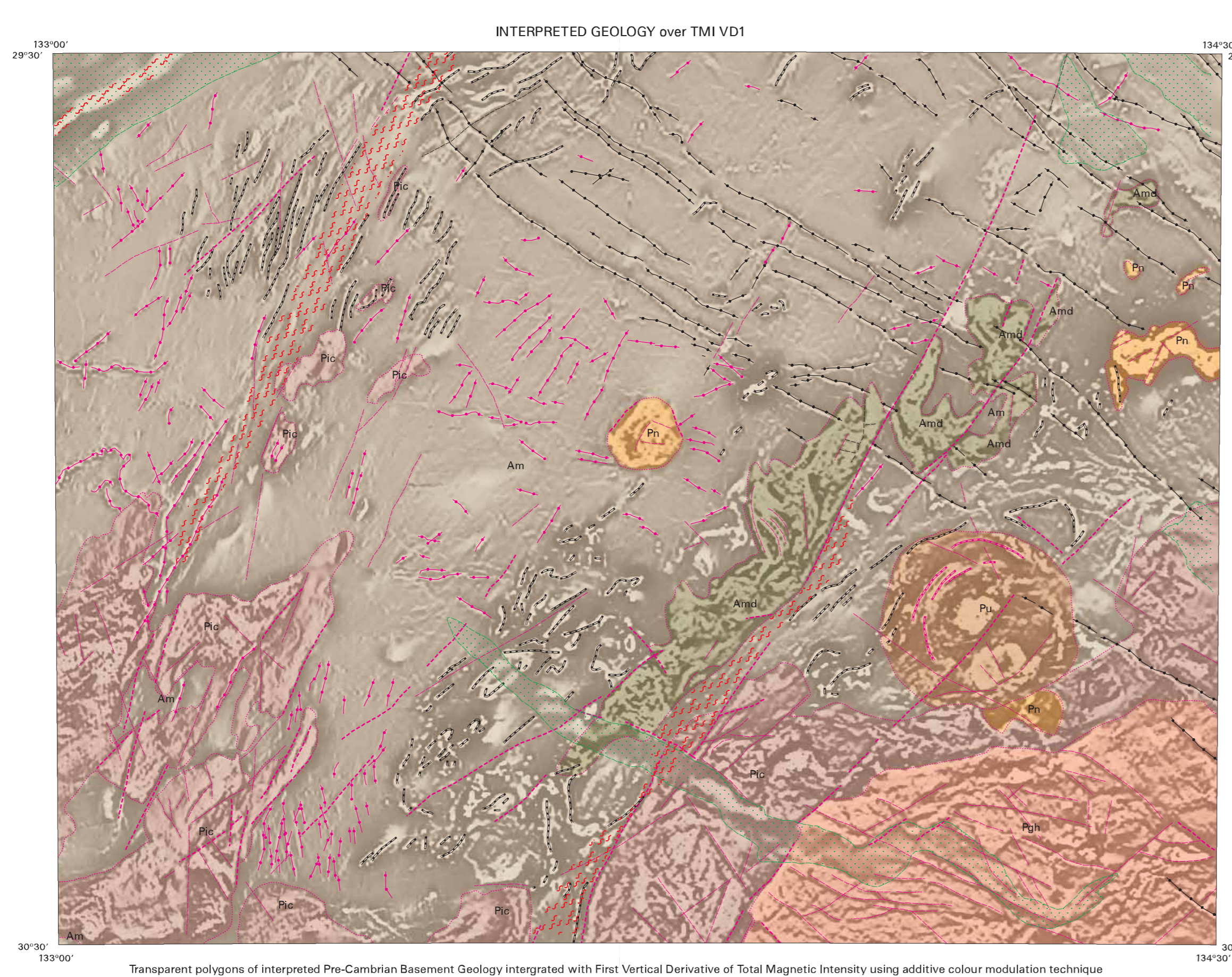
Transparent polygons of interpreted Pre-Cambrian Basement Geology integrated with First Vertical Derivative of Total Magnetic Intensity using additive colour modulation technique
