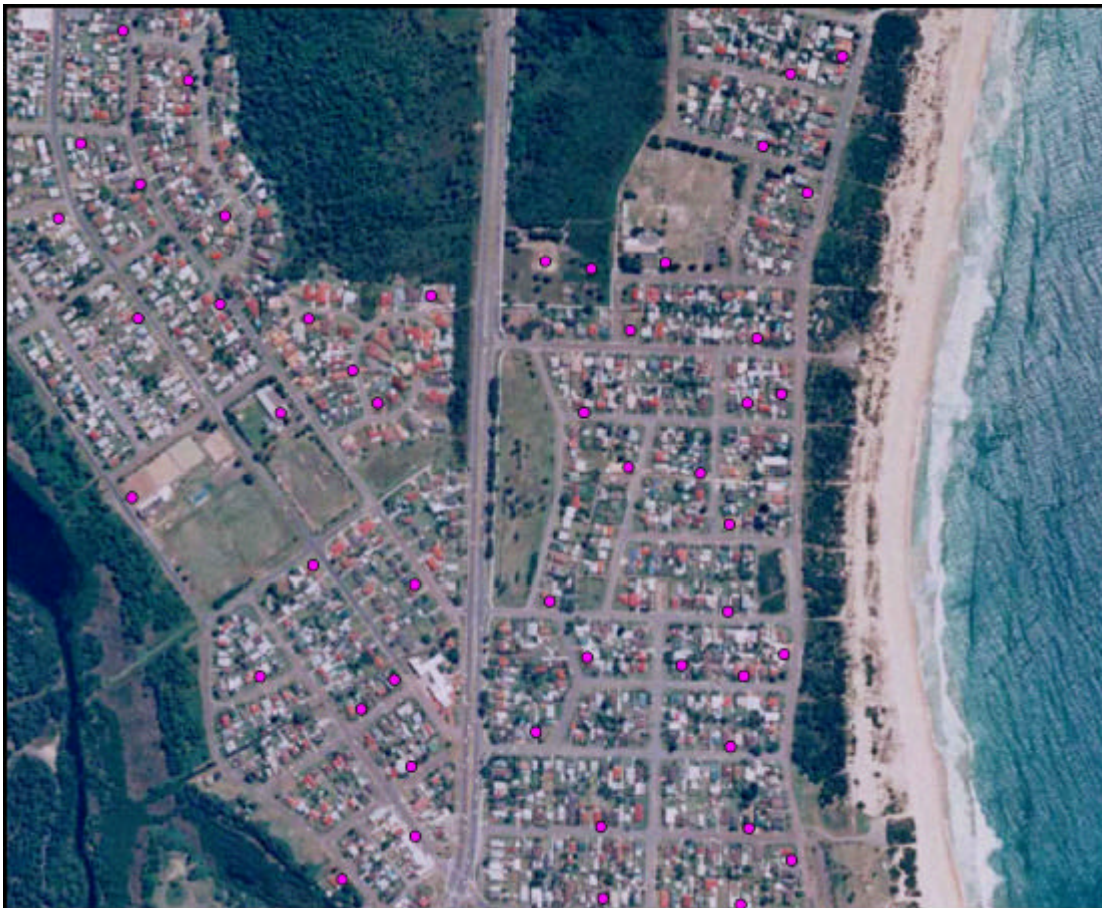
Figure H - 3: Aerial orthophoto of an area in Lake Macquarie with surveyed building points
