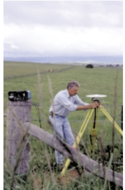
A surveyor at work. Precise positioning using geodetic GPS equipment of this type is routine in regional Australia for many surveying purposes.
