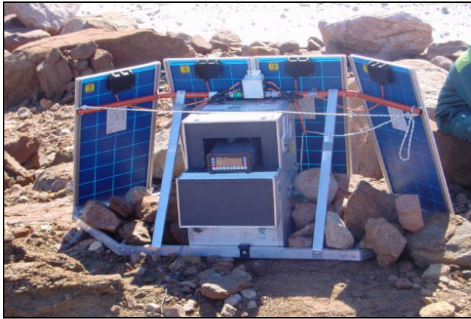
Figure 6.3.3 Solar Panel and GPS warm box set up at AUS351
