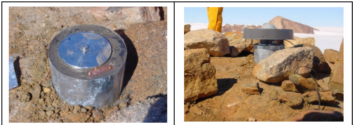
Figure 6.3.2 Photo of AUS351 Station Mark and GPS Choke Ring Antenna
