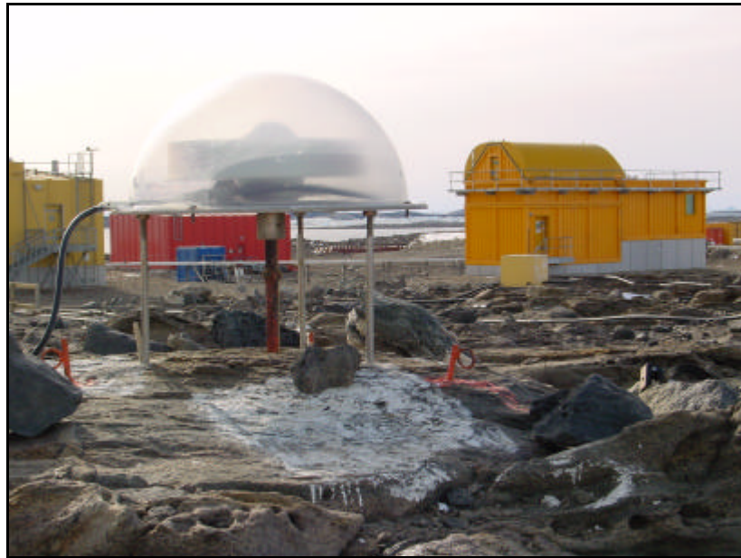
Figure 2.2.1 Photo of the ARGN Mark (AUS099) at DAVIS Station
