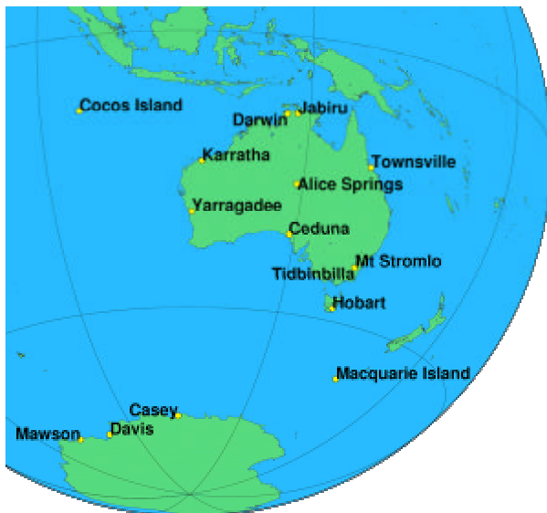
Figure 1. The Australian Regional GPS Network (ARGN). Consisting of 15 dual frequency geodetic quality GPS receivers tracking continuously.
