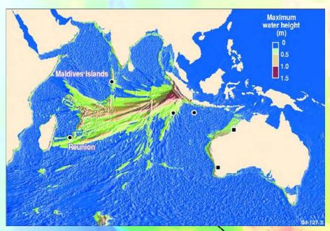
▲ Figure 2. Calculated maximum amplitude of the tsunami caused by 1833 Sumatra earthquake. Most tsunami energy was directed into the open Indian Ocean, away from the Bay of Bengal. (Numerical modelling performed by David Burbidge of Geoscience Australia.)
