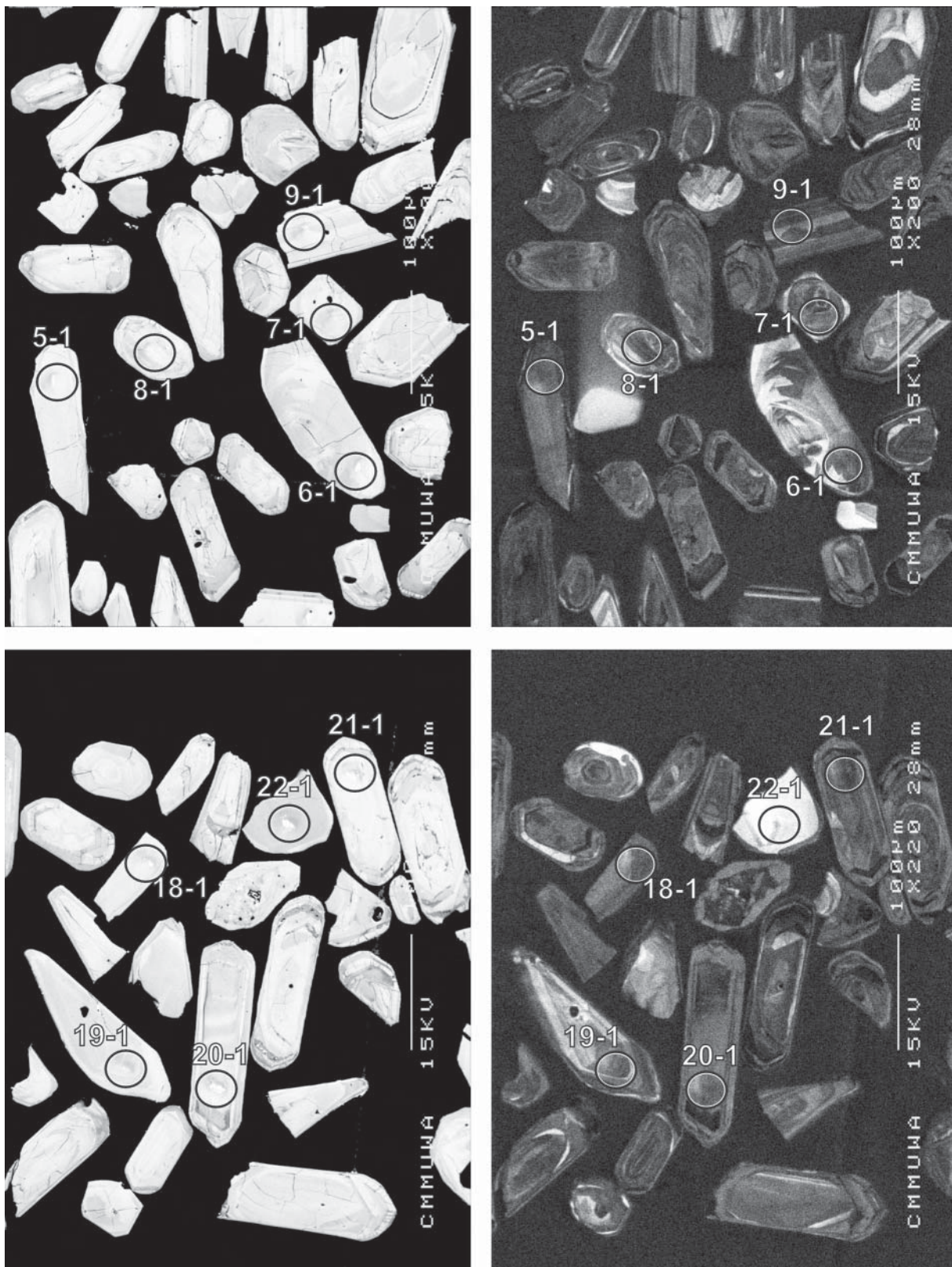
Figure 84. Representative SEM images (BSE on left, CL on right) for sample 2001969111B: gneissic biotite trondhjemite, Wingora Soak. SHRIMP analysis spots are labelled. Remnant pits from the ion microprobe analyses are faintly visible in some grains. Scale bar is 100 \mu\text{m} .
