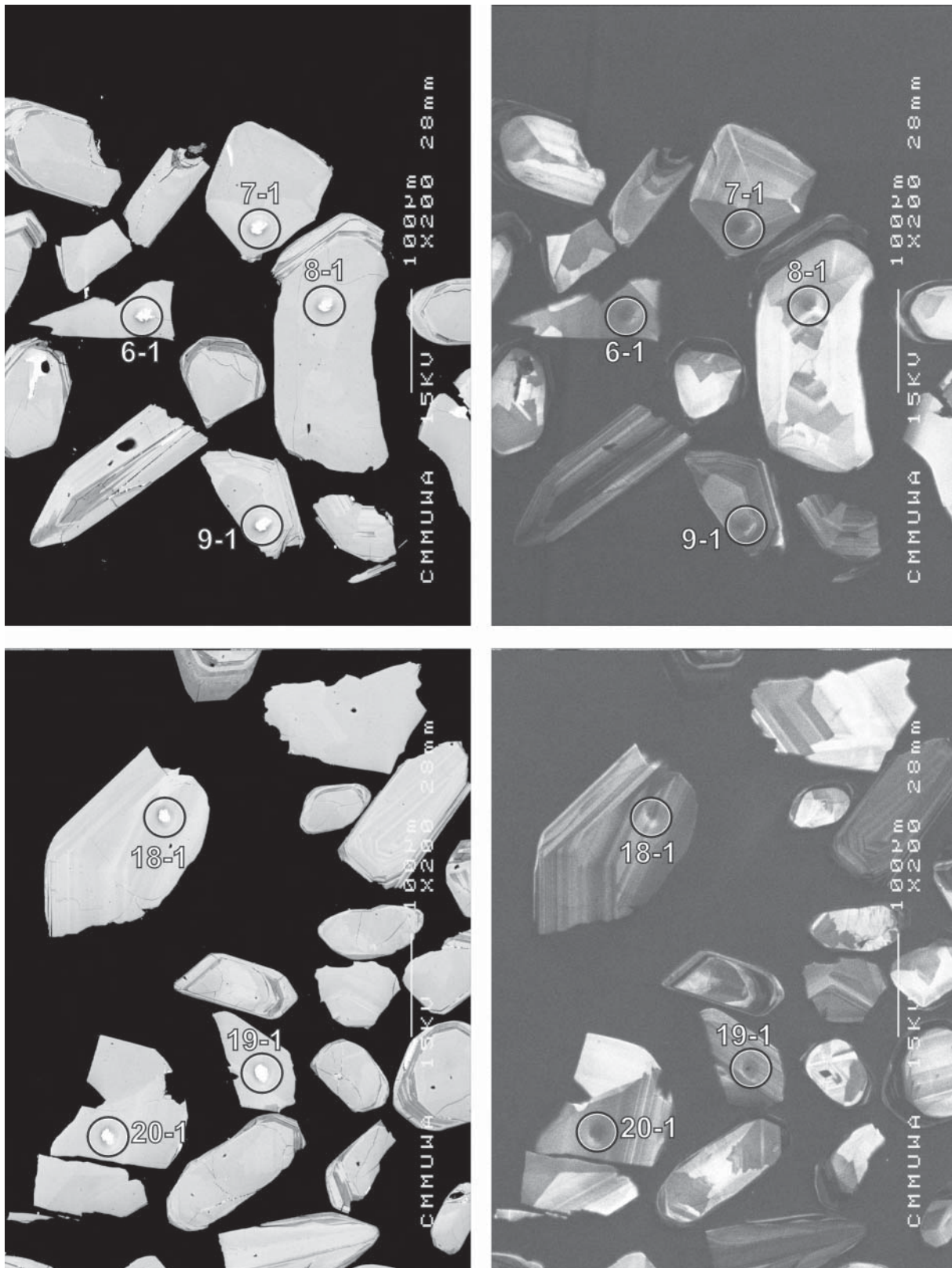
Figure 82. Representative SEM images (BSE on left, CL on right) for sample 2001969053C: banded biotite granitic gneiss, Turkey Well. SHRIMP analysis spots are labelled. Remnant pits from the ion microprobe analyses are faintly visible in some grains. Scale bar is 100 \mu m.
