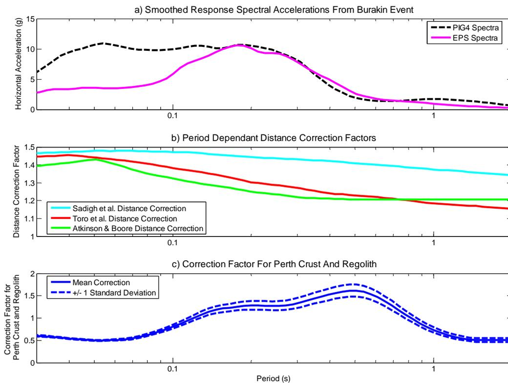
**Figure 5.21:** Data used for the development of a geological correction factor to account for the crust and regolith in the Perth study region. **a)** Response spectra recorded from the Burakin event. **b)** Period dependant distance corrections derived from Sadigh *et al.* (1997), Toro *et al.* (1997) and Atkinson and Boore (1997). **c)** Final correction including variability
