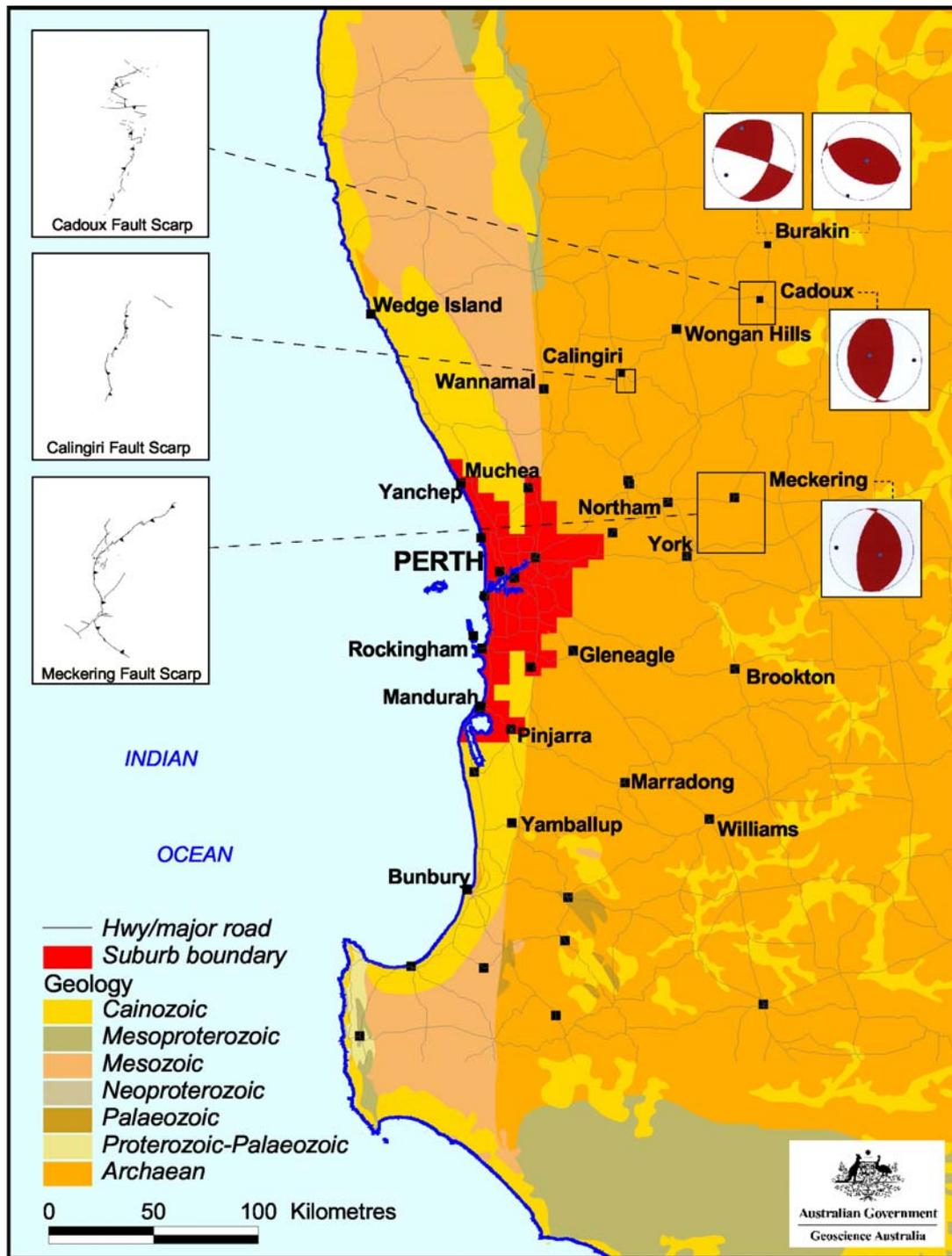
**Figure 5.7:** Geology of the wider Perth region showing fault scarps for the three largest earthquakes, Meckering, Cadoux and Calingiri. Fault plane solutions are shown for Meckering, Cadoux and the two Burakin 2001 earthquakes.
