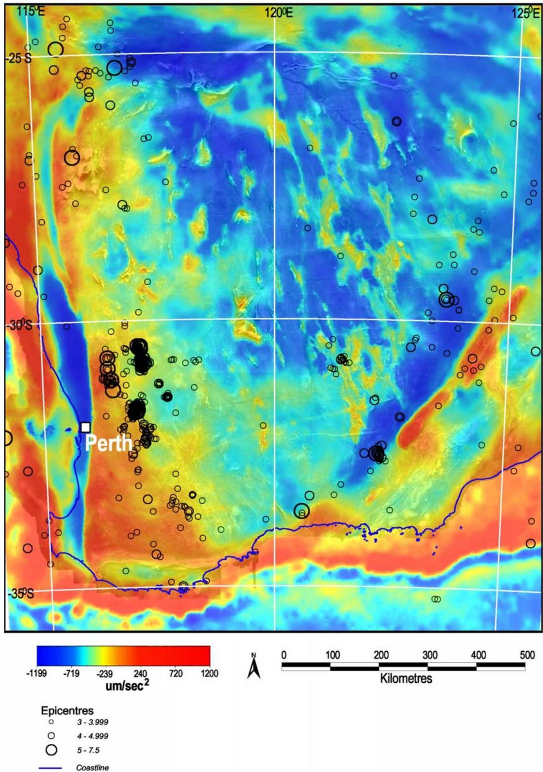
**Figure 5.4:** Combined gravity/magnetics image with seismicity (earthquake epicentres) for southwest WA. The Richter magnitudes of the earthquakes are indicated by the circle size as shown in the key.
