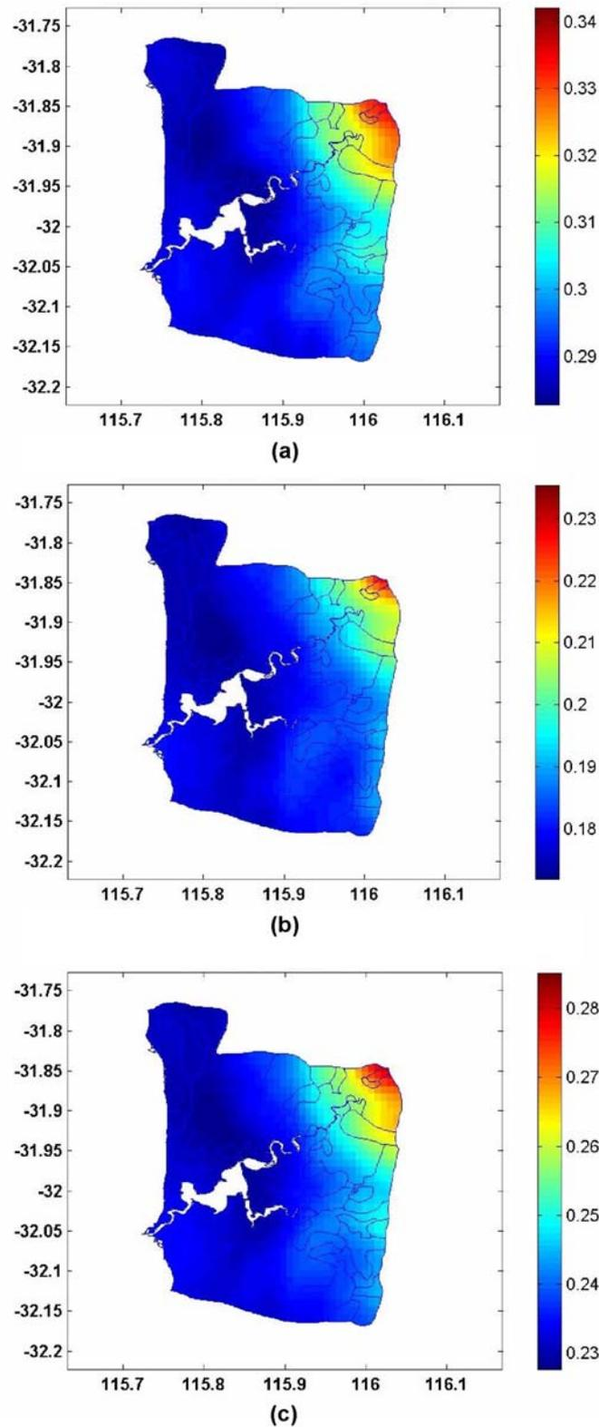
**Figure 5.15:** Earthquake hazard on rock in Perth with 10% probability of exceedence in 50 years,  $PGA(g)$ . **a)** Atkinson and Boore attenuation model results. **b)** Toro *et al.* attenuation model results. **c)** Combined with 50/50 weighting to the Atkinson and Boore model and Toro *et al.* model
