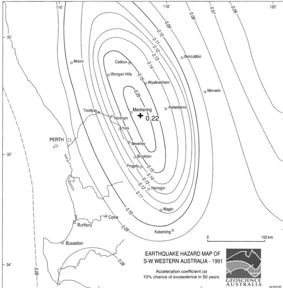
**Figure 5.14:** Earthquake loadings standard (Standards Australia, 1993) hazard map of WA
