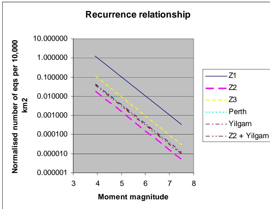
**Figure 5.9:** Recurrence relationship for the areal seismic zones
