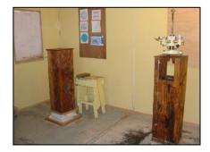
Figure 3. Inside the absolute hut—an Askania declinometer is mounted on the primary absolute pier.
