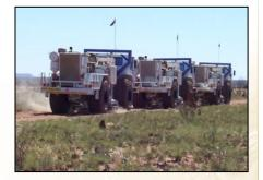
Figure 2. ANSIR (through Terrex Seismic Pty Ltd) seismic acquisition in operation in the Tanami with three IVI 60 000 lb vibrators operating on traverse 05GA-T2 to send signals through whole of crust and back.
