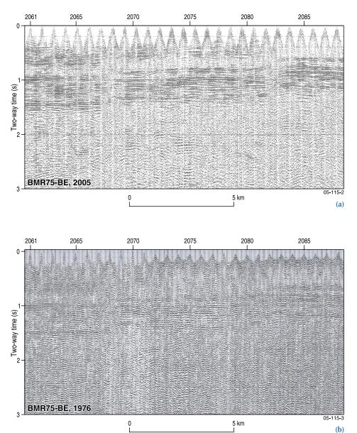
Figure 2. (a) 2005 reprocessed section of part line BMR75-BE, (b) 1976 vintage processing of part line BMR75-BE.
