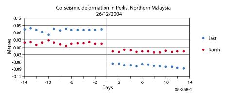
**Figure 1.** Co-seismic deformation at GPS site ARAU (Perlis, northern Malaysia).
