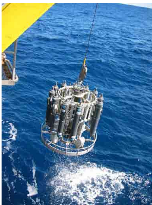
Figure 4.1. Photograph of CTD rosette deployed from starboard A-frame. Niskin bottles were attached to the rosette to collect water samples from near the bed and at the surface.
