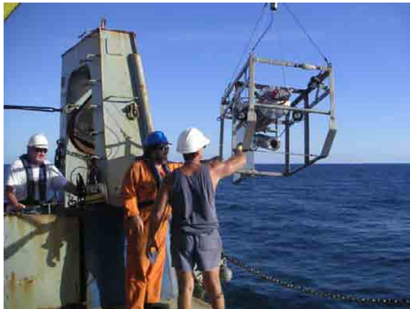
Figure 4.2. Photograph of the underwater digital video camera system. The camera provides broadcast quality digital video. The camera and lights are powered from the surface and a live video feed is transmitted to the vessel.
