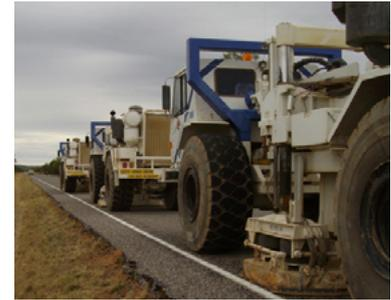
**Figure 2.** Seismic vibrator trucks operating between Croydon and Georgetown, northwest Queensland.
