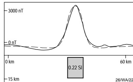
Fig. 17. An example of modelling the large magnetic anomaly over the greenstone belt in Figure 16 (q.v. for location of profile). Observed profile, continuous line; modelled profile, dashed line.
