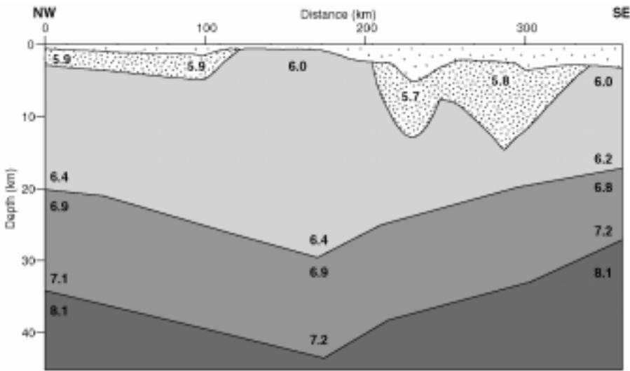
Fig. 23. The P-wavespeed model derived from the seismic arrival times along the Broken Hill profile.
