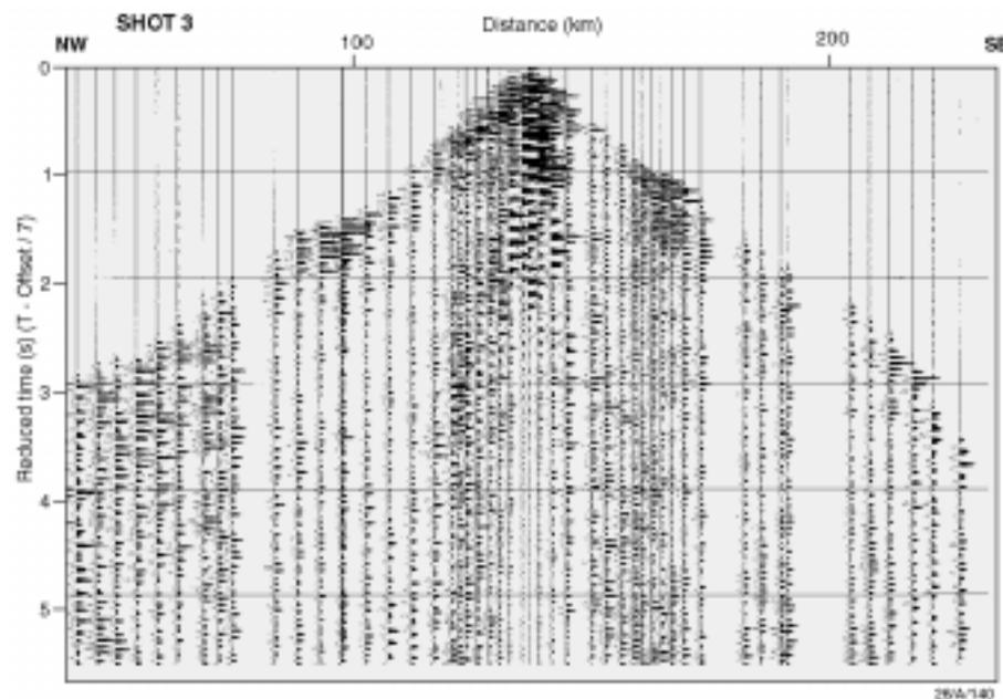
Fig. 21. An example of the Pg1 arrivals from shot 3 detonated north of Broken Hill and recorded across the Broken Hill Block. These Pg1 arrivals show little delay time, indicating the presence of basement rocks with a P-velocity near 5.9 km/s near the surface.
