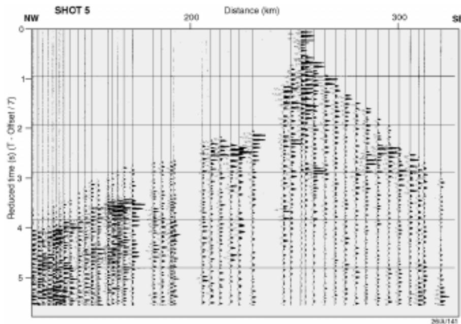
Fig. 22. An example of the Broken Hill survey Pg1 arrivals from shot 5, detonated east of Menindee. These Pg1 arrivals show a significant delay time, indicating the presence of near-surface low-velocity rocks. The striking asymmetry of the Pg1 arrivals indicates rapidly changing geometry of this low-velocity zone, which corresponds to the Menindee Trough.
