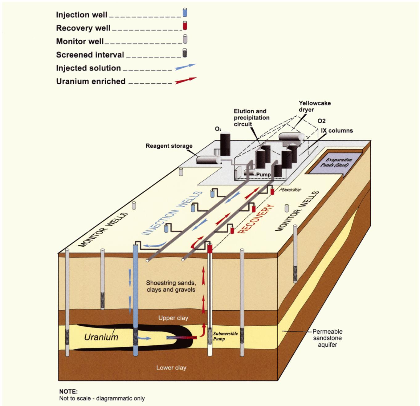
**Figure 2.** Schematic block diagram of in situ leach uranium mine, based on figure from the Beverley EIS (Heathgate, 1998).
