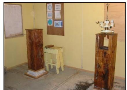
▲ **Figure 3.** Inside the absolute hut—an Askania declinometer is mounted on the primary absolute pier.
