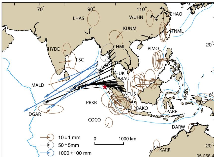
◀ Figure 2. Displacement field for the earthquake region determined by GPS. The red star represents the epicentre, and the green lines show plate and fault boundaries.
