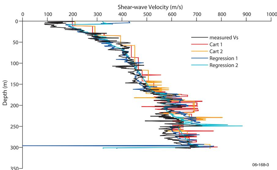
▲ **Figure 3.** Comparison of predicted shear-wave velocity for various models against measured  $V_s$  from a reference site from Long Beach, California.
