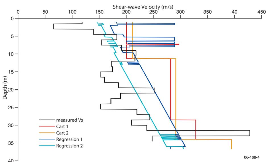
▲ **Figure 4.** Comparison of predicted shear-wave velocity for various models against measured  $V_s$  from a reference site from Newcastle, Australia.
