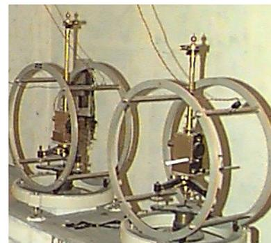
**Figure 2.** Gngangara's recording vault, showing the historic Eschenhagen equipment. The Eschenhagen variometer was first installed at Watheroo observatory by the Department of Terrestrial Magnetism in 1919. It was transferred to Gngangara in 1960 and operated there until 1991. This historic equipment is now on display in the Geoscience Australia building foyer.
