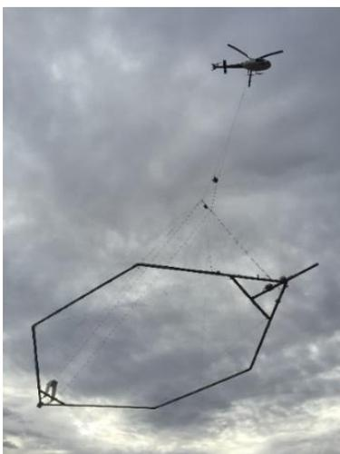
Figure 1. Helicopter AEM system with an antenna frame.
