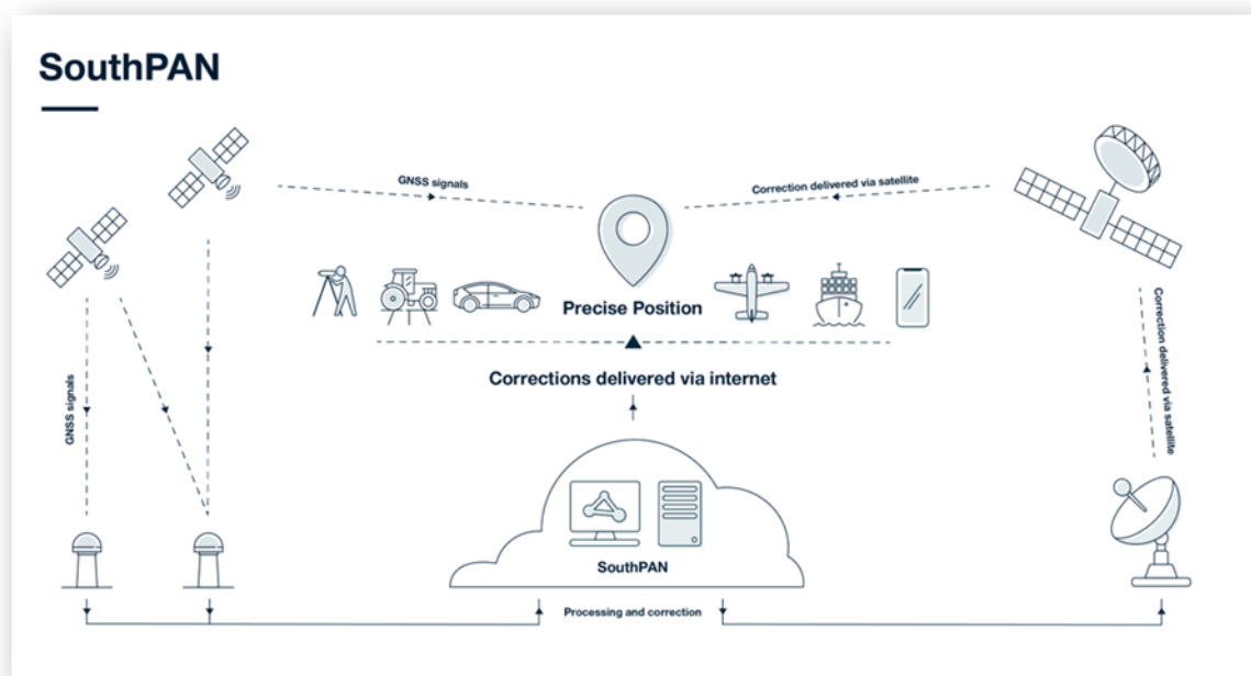
Figure 2: SouthPAN System Architecture
