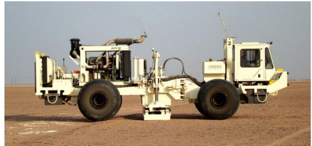
A picture of a Vibroseis truck. The vibrating plate can be seen in the middle of the truck in contact with the ground.
