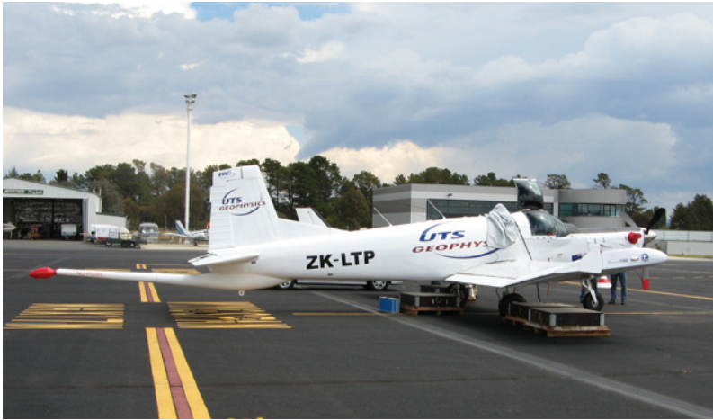
Figure 2. UTS' highly modified Fletcher aircraft, purpose-built for the slow, low level survey flying required by AWAGS 2.
