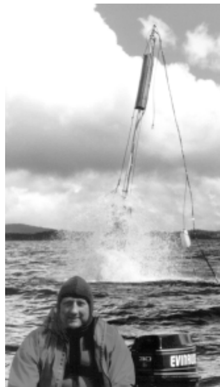
Fig. 10. AGSO's Mackereth lake-bed corer surfacing in Great Lake behind Professor Eric Colhoun.
