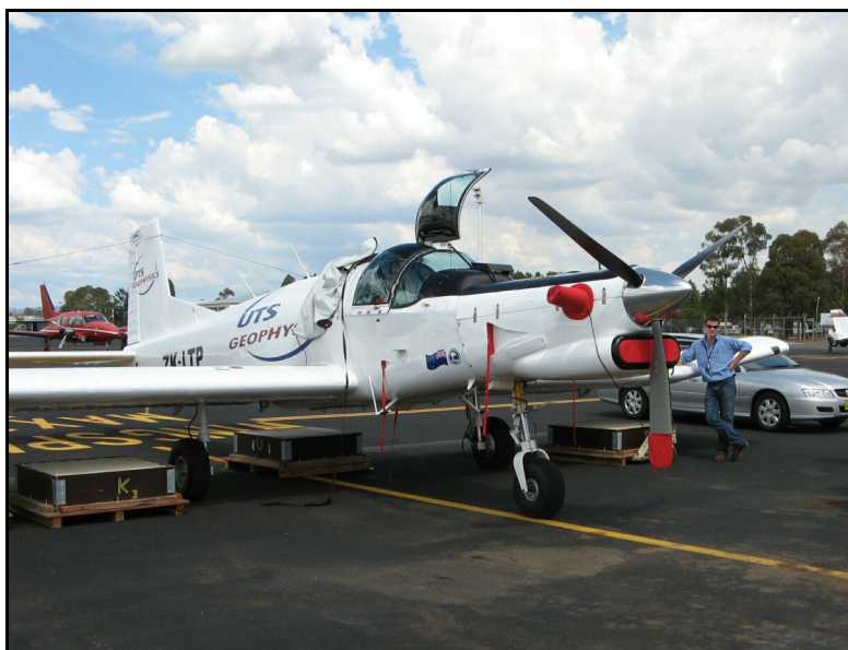
Figure 2: The Cresco survey aircraft used by UTS Geophysics to fly the AWAGS survey, undergoing spectrometer calibrations at Canberra airport.
