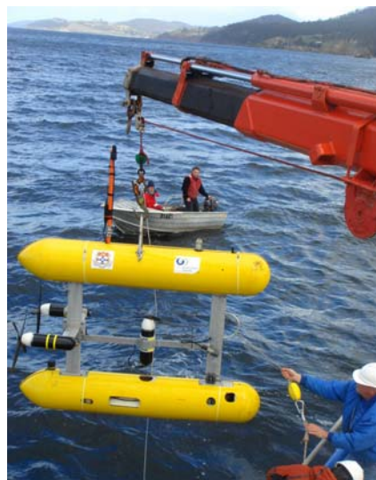
Figure A.1: Deployment of Autonomous Underwater Vehicle Sirius from R.V. Challenger .
