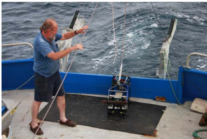
Figure 1.5: RayTech small towed-video system being deployed from the stern of RV Challenger .
