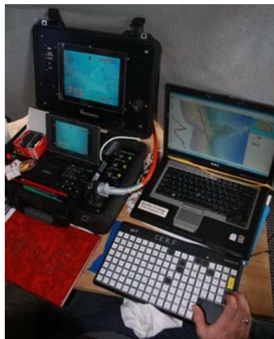
Figure 1.6: Real-time video display of underwater towed video (left), GPS navigation display and keyboard used for habitat characterisations of reef and surrounding areas.
