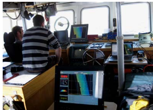
Figure 1.4: Wheelhouse of RV Challenger showing the EM3002 operator display (foreground) and the helmsman display on the bridge.
