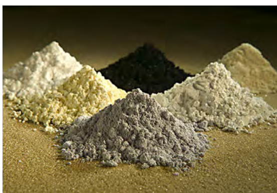
Figure 1.5. Rare-earth oxides that are used as chemical tracers to determine which parts of a watershed are eroding. Clockwise from top centre: praseodymium, cerium, lanthanum, neodymium, samarium, and gadolinium. Reproduced with permission (PD-USGOV-USDA-ARS) from the United States Department of Agriculture, Agricultural Research Service, at http://www.ars.usda.gov/is/graphics/photos/jun05/d115-1.htm Group Elements (red font). Modified from Haxel et al. (2005).
