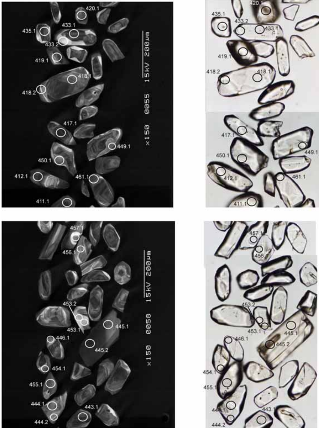
Figure 82. Representative CL (left) and transmitted light (right) images for sample 200236 8028b: leucogabbro, Mt Woods Inlier. SHRIMP analysis spots are labelled. Scale bar is 200 \mu\text{m} .
