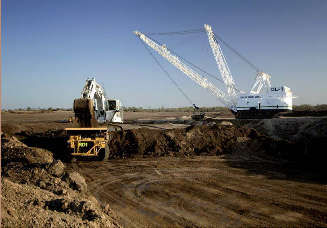
Overburden removal at the Rolleston mine, Queensland (Xstrata Coal Australia Pty Ltd).
