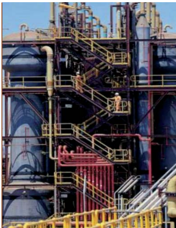
Pulse columns at uranium processing plant, Olympic Dam, South Australia (BHP Billiton Ltd).
