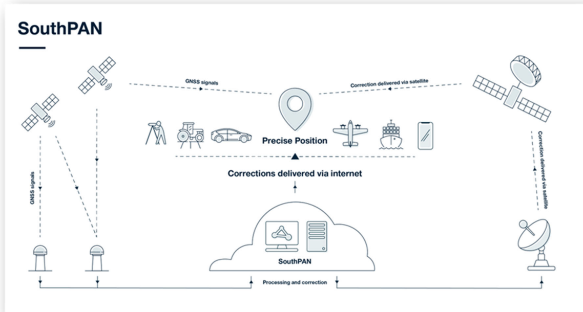
Figure 2: SouthPAN System Architecture
