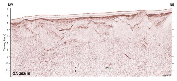
Figure 2. Profile along Line 19 of the S302 seismic survey, revealing a number of sediment-filled depocentres. The line location is shown in figure 1.
