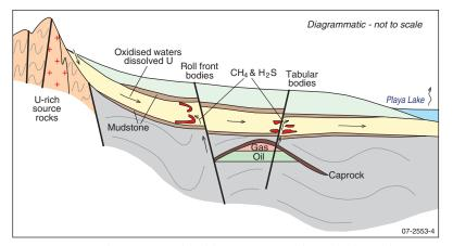
**Figure 4.** Diagrams showing proposed model. Uranium is carried in oxidised groundwaters and reduced by hydrocarbons and/or  $H_2S$  released from the underlying oil and/or gas field. Both roll-front and tabular ore bodies can result from the process. During ore deposition hydrocarbons are often oxidised to form carbonates.
