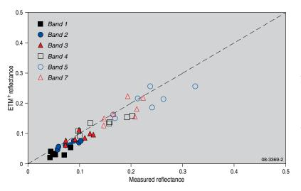
**Figure 2.** Comparison of Landsat-derived surface reflectance values with field measurements obtained in June 2008, Gwydir River catchment. Reflectance is measured for wavelength band for each pixel.
