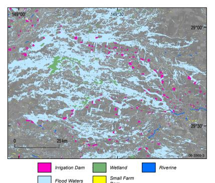
Figure 3. Water body map of Gwydir River catchment generated by aggregating and classifying minimum reflectance values in Band 5 from a stack of cloud-free Landsat images acquired in 2004.
