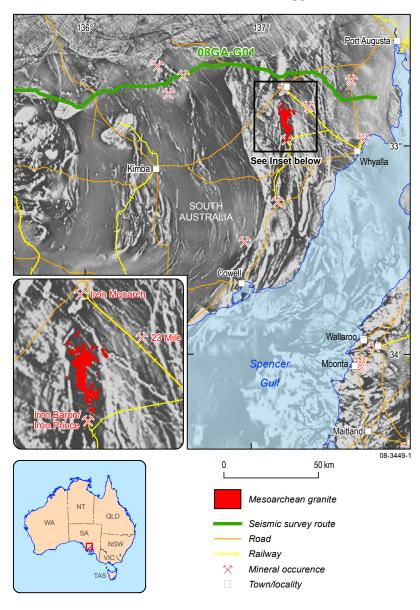
**Figure 1.** Magnetic image of the northeastern Eyre Peninsula showing the trace of the recently collected seismic line (bold green line), and the location of Mesoarchean granite (highlighted in red) between the Iron Monarch and Iron Baron mines (inset).
