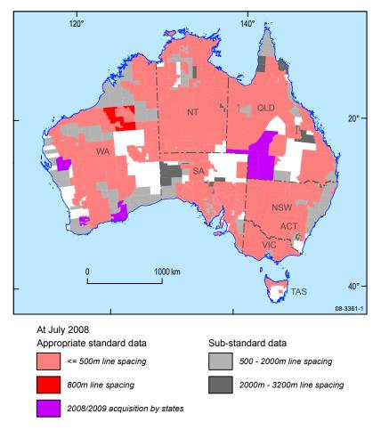
**Figure 1.** Radiometric data acquisition by Geoscience Australia and state and Northern Territory geological surveys.
