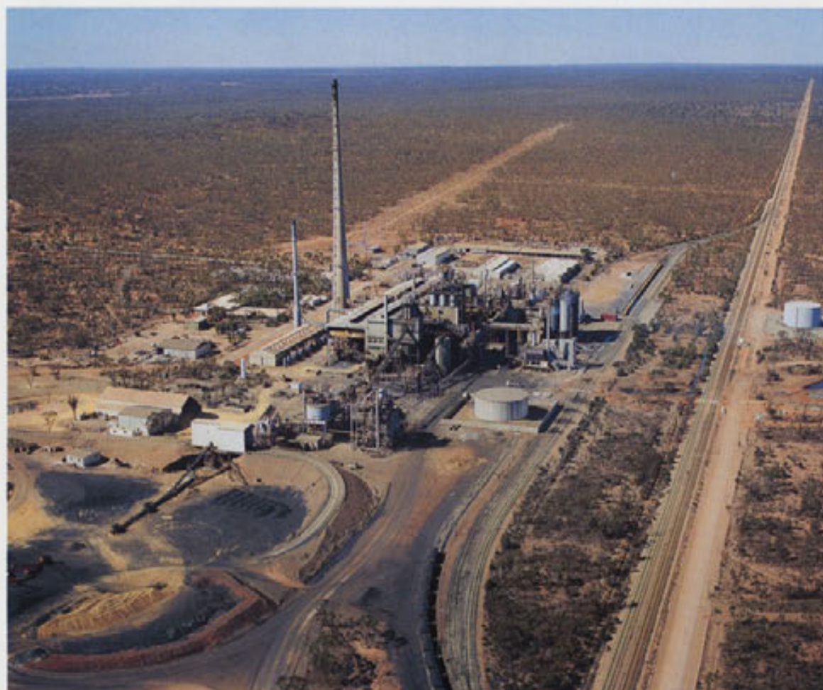
Australia's only nickel smelter, near Kalgoorlie (W.A.) Concentrates from surrounding nickel mines are smelted at the Kalgoorlie nickel smelter. Each year the smelter produces around 73 000 t of granulated nickel matte which is railed to Kwinana for refining or export.
