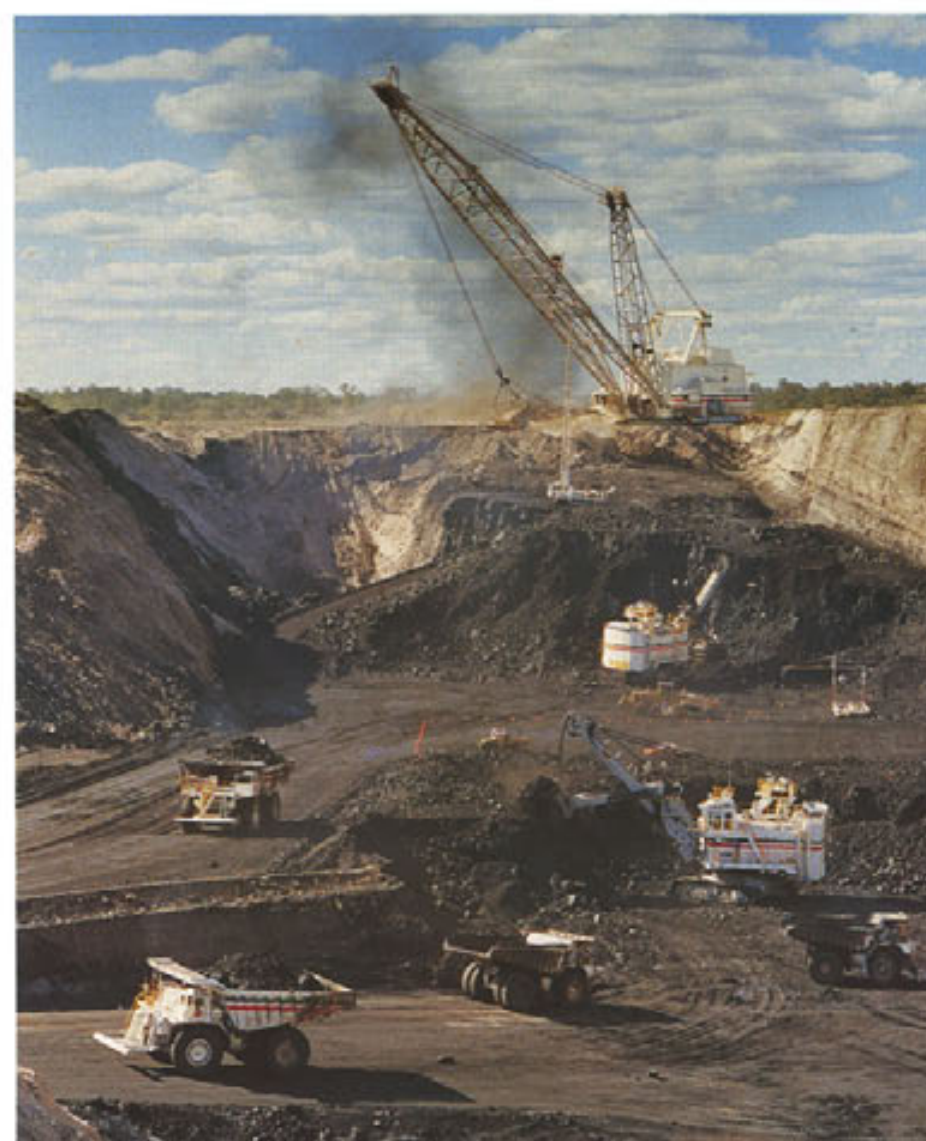
Mining the 30-metre thick black coal seam at Blair Athol, central Queensland Over 5 million tonnes of steaming coal is produced annually by strip mining at Blair Athol. Most of the coal is railed nearly 300 km to Dalrymple Bay for export. The shallow overburden is removed by a 46 m 3 capacity dragline to expose the unusually thick coal seam.
