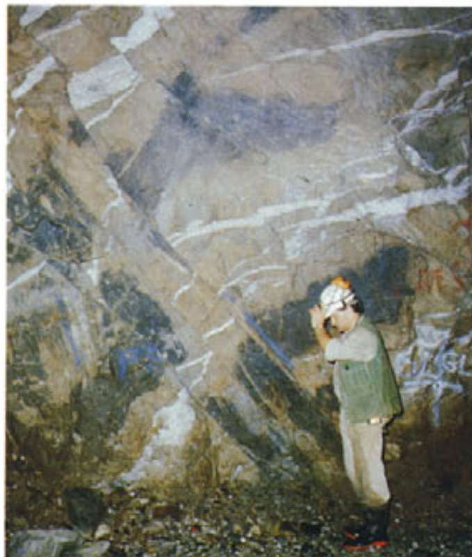
Strongly mineralised Archaean dolerite, Mount Charlotte gold mine, Kalgoorlie (W.A.) Gold is associated with the altered paler rock surrounding the white quartz veins.
